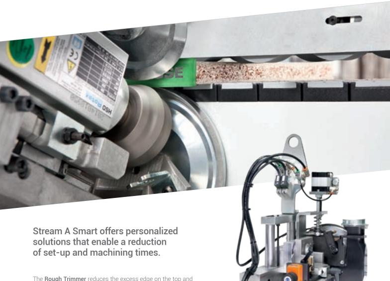
The **Rough Trimmer** reduces the excess edge on the top and bottom of the panel. It guarantees a perfect finish for solid wood, in one single movement.
